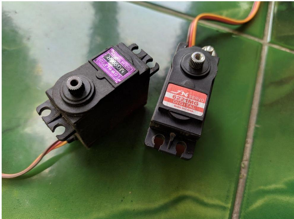
Gambar 2.6 motor *servo* MG966R
