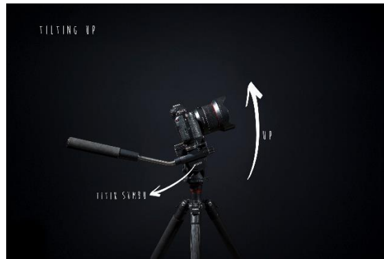
Gambar 15 . Contoh tilt up & tilt down ( Sumber : overloop.com )
