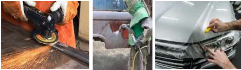
Gambar 35. Proses Operasi Permukaan (Surface processing operations): a) Pembersihan (cleaning): Proses Grinding; b) Perlakuan permukaan (Surface treatments): Proses Sand Blasting; c) Proses pelapisan dan deposisi film tipis (Coating and thin film deposition): Proses Coating Film.
