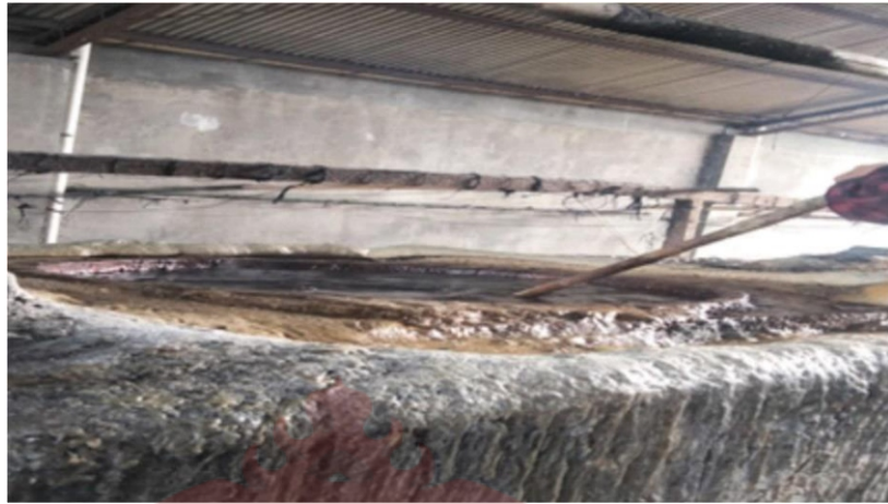
Gambar 15. Proses Pelorotan Malam Sumber (Foto Safitri Nurjannah, 2024)
