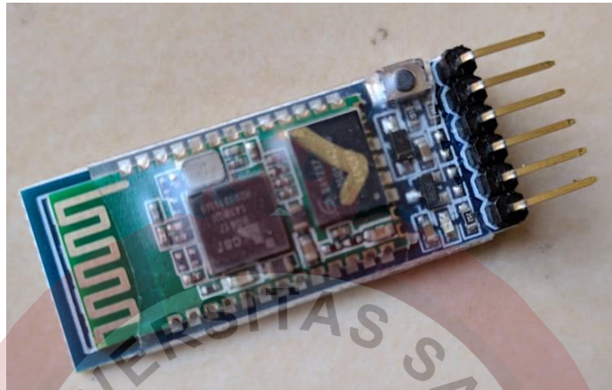
Gambar 2.5 Modul Bluetooth HC-05
